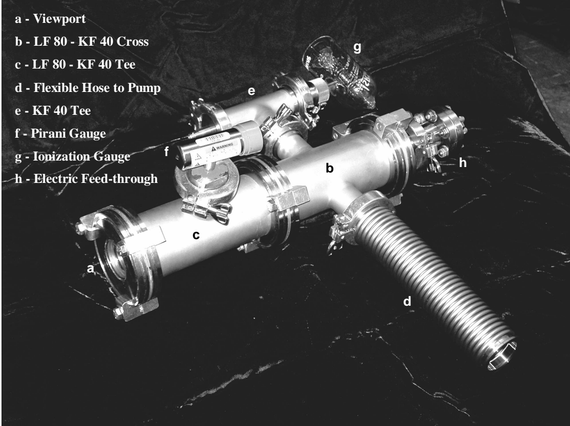
Figure II. 1 - Modular vacuum chamber used in most x-ray, electron, and ion emission experiments.
