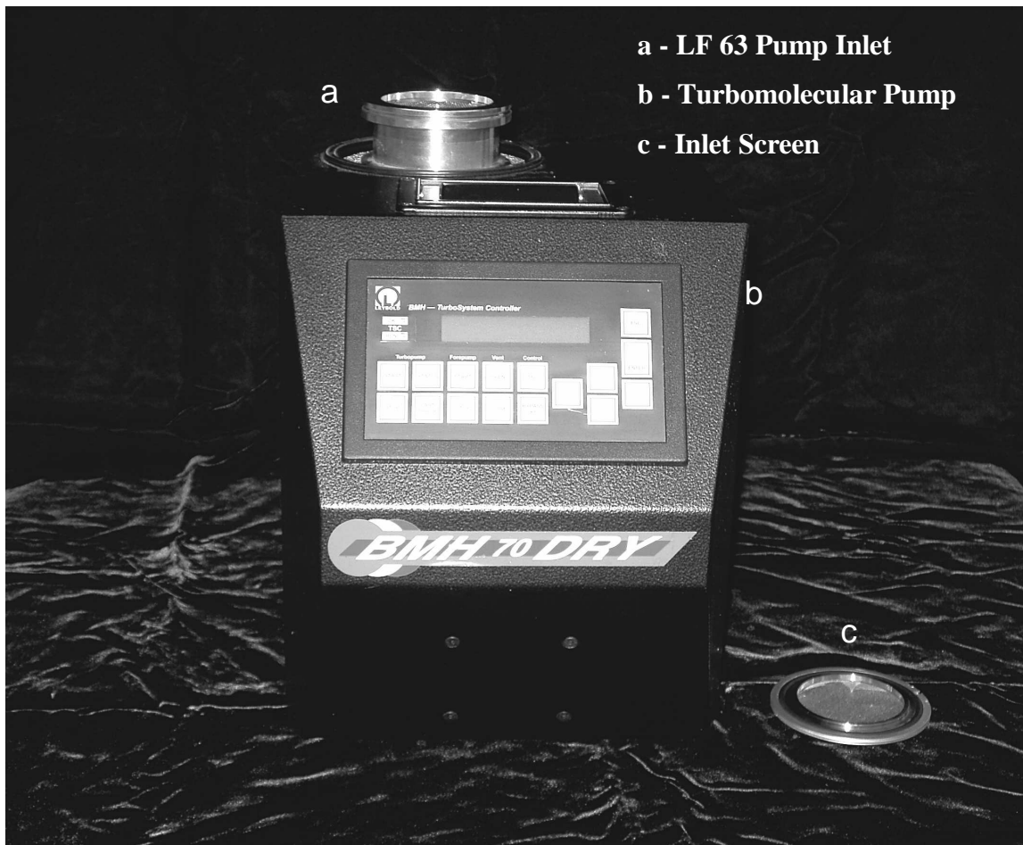
Figure II. 5 - Leybold BMH 70 DRY turbomolecular vacuum pump used in the pyroelectric neutron production experiments. The vacuum chamber was attached to the LF 63 pump inlet.
